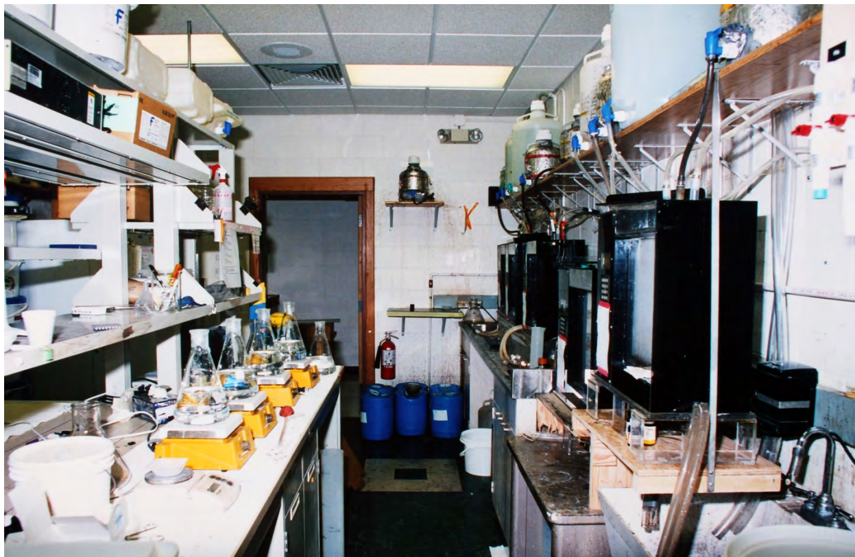
Silver staining room (2000). At the peak of SSCP mutation detection and STRP genotyping, the lab electrophoresed and interpreted forty 60-lane gels per day (2400 PCR reactions).
