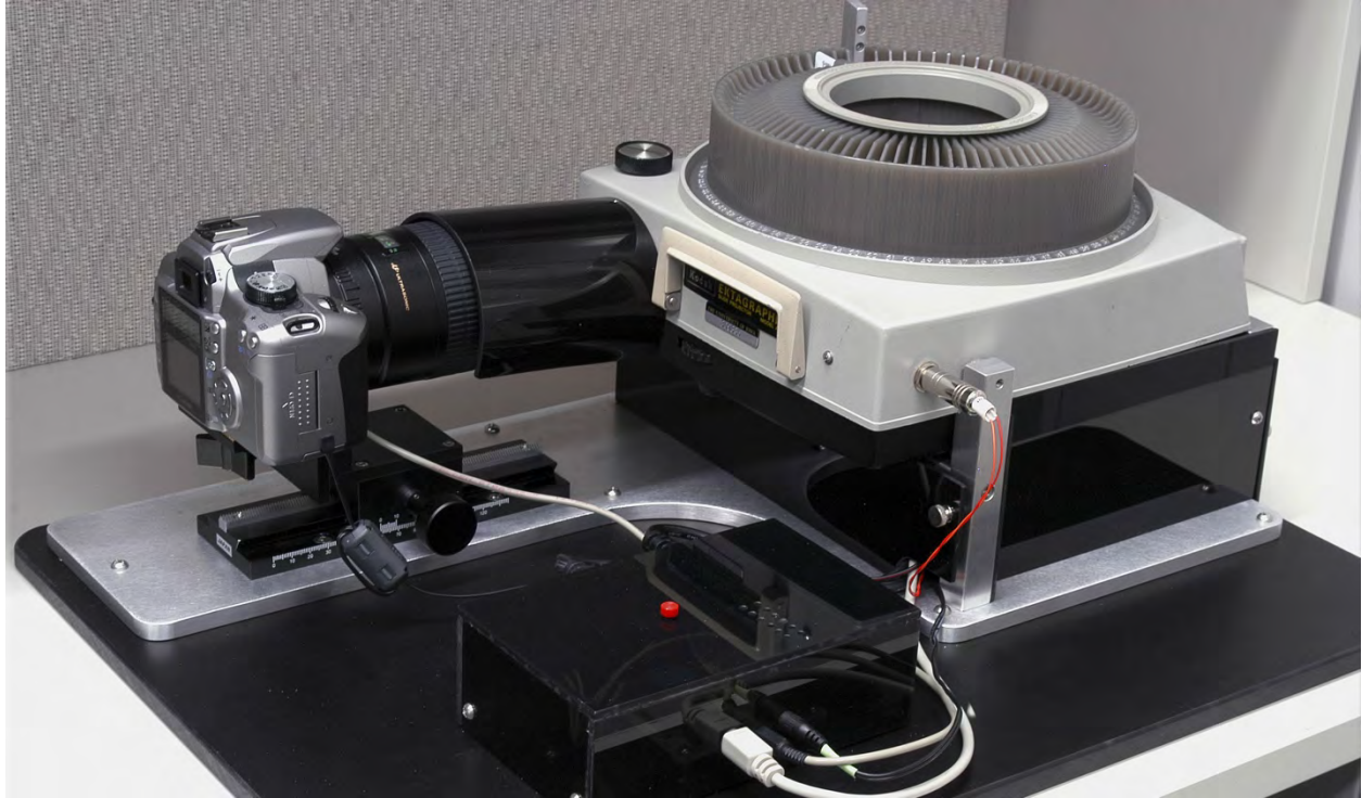
High-throughput 35 mm slide digitizing device. The greatest challenge of digitizing the tens of thousands of mounted 35mm slides in the department's photofile collection was mechanically handling slides of various ages and thicknesses without jamming. The Kodak carousel projector has the lowest jam rate of any slide handling device ever made. These projectors were fitted with a white-balanced LED light source and a 35 mm camera to digitize the entire inherited retinal disease collection of the department dating back to the early 1960s.
